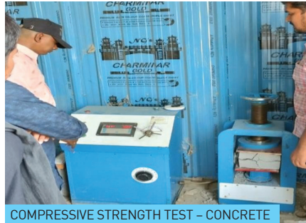
COMPRESSIVE STRENGTH TEST - CONCRETE
