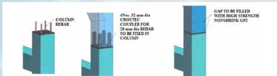
Fig: Erection Sequence at H-Frame to Pi-Frame Connection.
