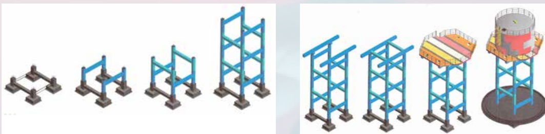
Fig: Representing Step by Step Development of Pre-Cast Overhead Tanks.
