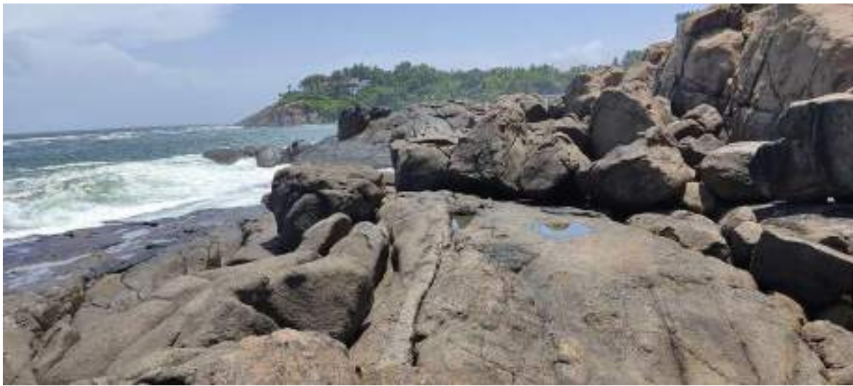
Figure 8-3 Representative field photographs of the massive charnockite with multiple joints and fractures at Edakkal/ Mid- rock, Kovalam.
