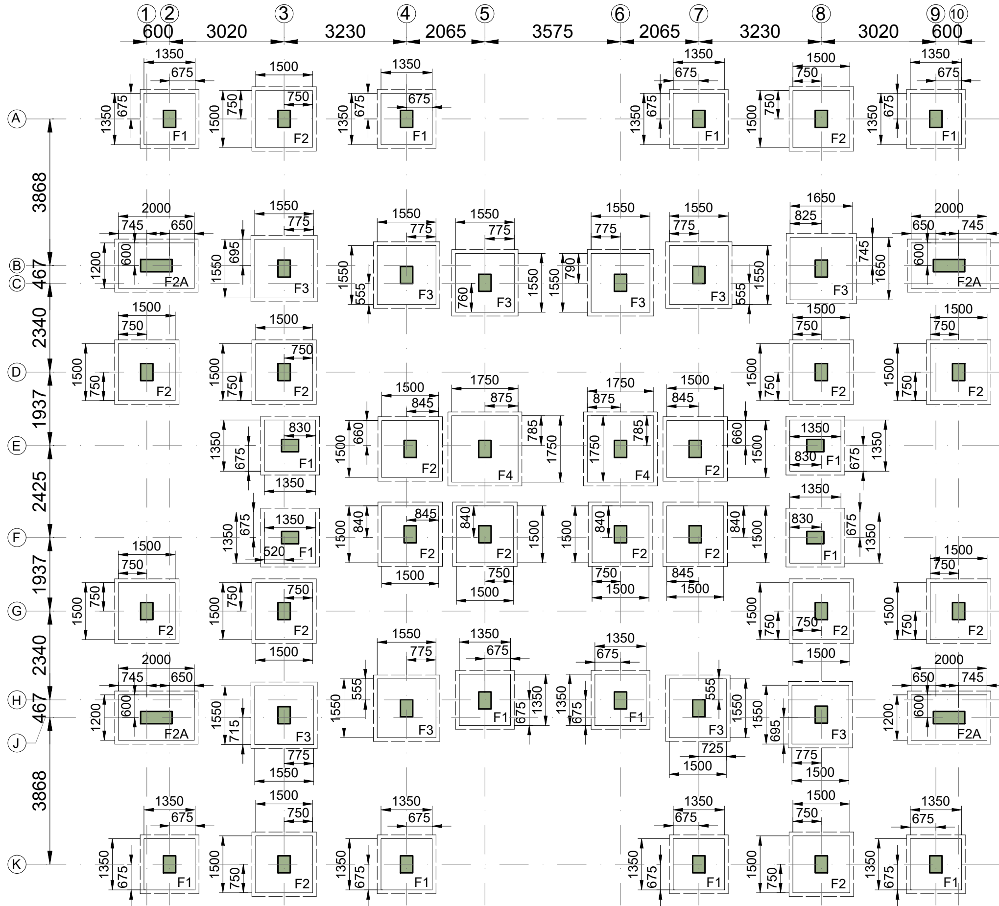
TYPE-II QUARTER FOUNDATION LAYOUT PLAN SCALE 1:100
